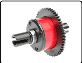
C-00180-685-1 Centre Diff Assembly - Alu/Steel - 52T - 100K Oil Filled - 1 Set
